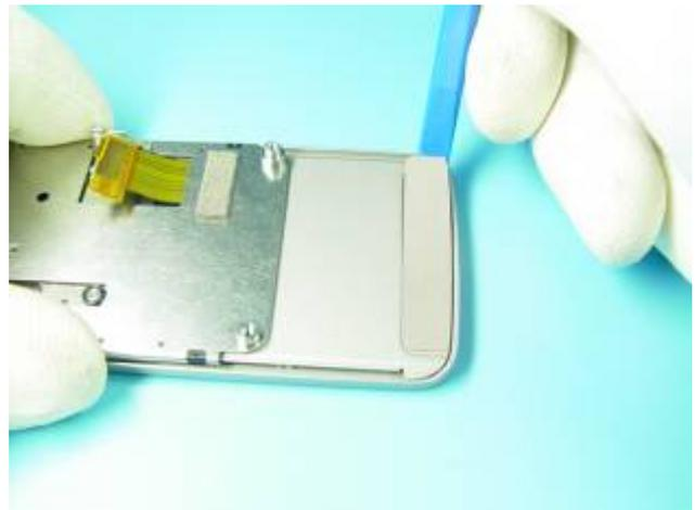
18) Peel off the Back Plate with SS-93.
